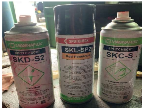
Gambar 4: Remover (SKC-S), Penetrant (SKL-SP2), Developer (SKD-S2).
